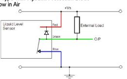
N-Type with Internal 10kΩ Pull-Up Resistor High in Air
