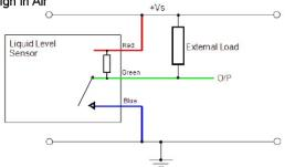
N-Type with Internal  $10k\Omega$  Pull-Up Resistor
